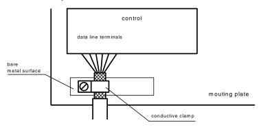
The cable shielding is to be connected at both cable ends. If equipotential bonding currents are expected due to the cable arrangement, electrical isolation is to be performed on one side. In this case, capacitive connection (approx. 0.1µF/600 V AC) of the shielding on the isolated side must occur.
