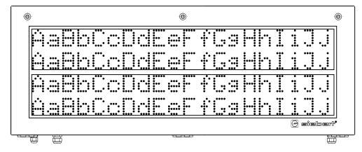
The physical distance between the matrix modules corresponds to a height of two pixels. Thus the distance between the first and second lines is the same as between the second and third lines.
